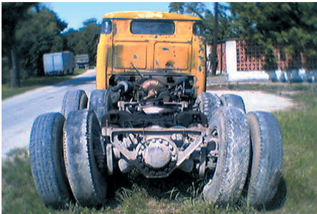
Fig. 3.25. Tatra truck: wheels are installed at an angle
