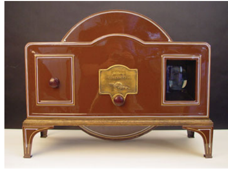
Fig.5.17. A TV-set having a Nipkow disk (the window on the right is a small screen)
