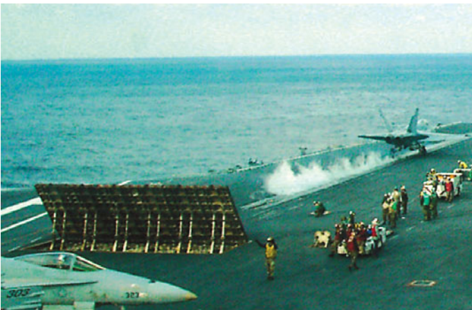
Fig. 6.6. An aircraft is taking off from an aircraft carrier (there is an impingement plate seen behind the aircraft)
