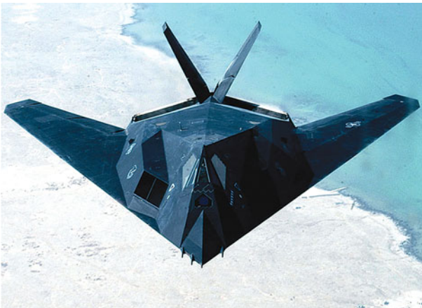
Fig. 3.33. The angular shape of a stealth aircraft F-117 dissipates radar beams Example: Aircraft shape
