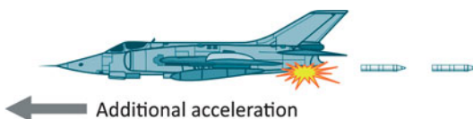
Fig. 6.4. Firing tail cannons accelerates the aircraft
