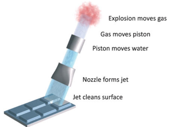
Fig. 6.63. Building a functional chain
