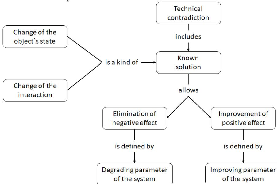
Fig. 5. Diagram for definition of the technical contradiction concept
