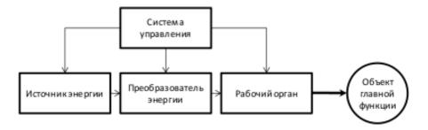
This diagram shows almost explicitly the energy flows from the source to the inverter and on to the actuator, and the information flows from the control system.
